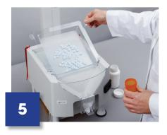
**Dispense -** Press Finish button to record the transaction, then lift platter to slide pills into funnel.
