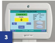
**Verify** - Eyecon will proceed to count mode if Rx label matches the stock bottle. Eyecon will display error if mismatch is detected.
